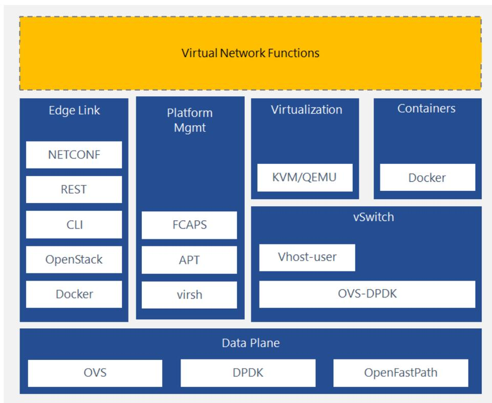
Figure 5. Open Architecture in the NFV Access Design
