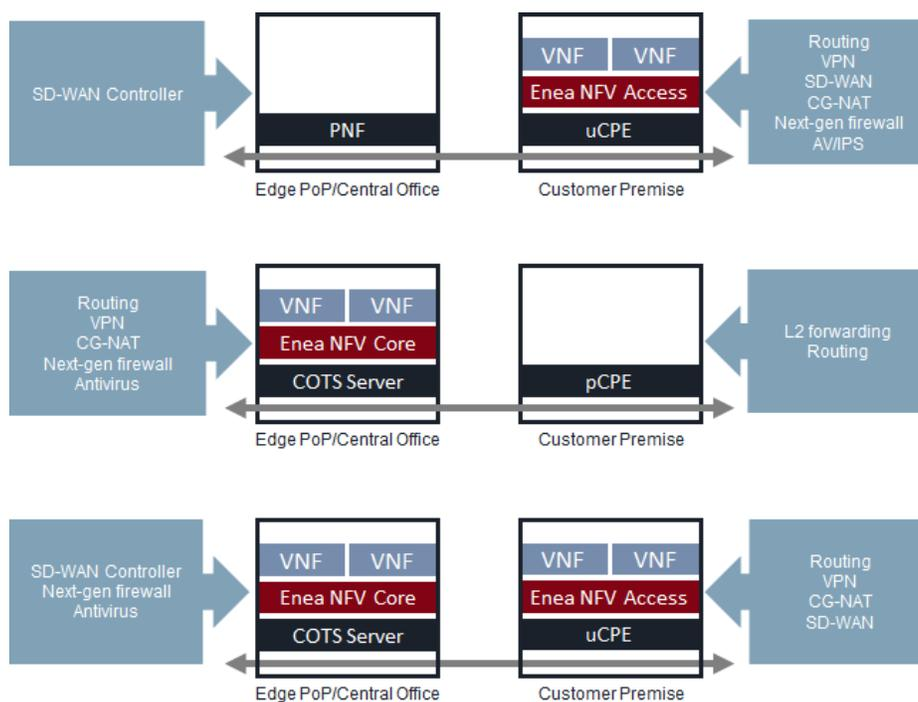
Figure 4. Flexibility in Deployment Options with NFV Access and Core
