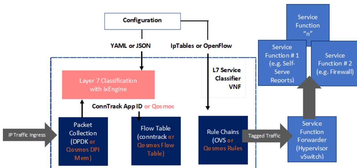
Figure 2. L7 Based Service Chaining Based on Enea Qosmos ixEngine
