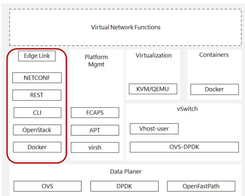
Figure 1. Edge Link Functions for Open, Standards-Based Management of NFV-Based Services at Scale
